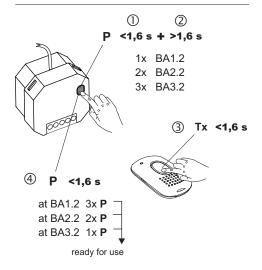
Р programming button dimmer transmitter button Tx
